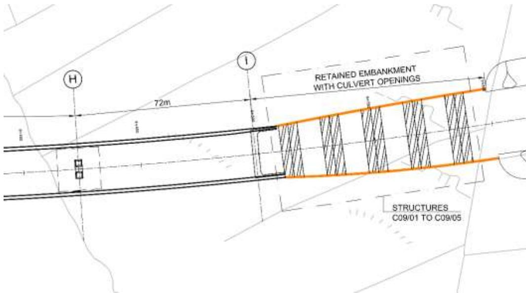
**Figure 2.12: Elevation of Retained Embankment Tie-in**
